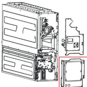
2. Disconnect the condensate pump (CN13) and water level switch (CN5) from the indoor unit's main board.
