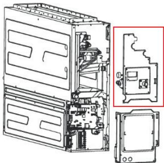
4. Remove the 4 screws circled in red and rotate the pump assembly 90 degrees. Reinstall the screws.
