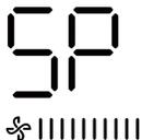
When the air conditioning unit is off, into the query function of temperature, press " ^ " or " v " to select SP, press "Confirm" to adjust the static pressure value.
