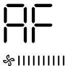
When the air conditioning unit is off, into the query function of temperature, press " ^ " or " v " to select AF, press "Confirm" into test mode and flash "ON", press "Back" or press "ON/OFF" or press "Confirm" drop out of test mode. In AF mode, 3~6 minutes test completion automatically exits. When it exits, it should no display "ON", if the test process, press "Back" or press "ON/OFF" or press "Confirm", the test exits will be interrupted.
