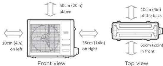
Note: Outdoor units must be elevated 30.5-61cm (12-24in.) above the surface below in heating applications to allow for snow clearance and defrost runoff. Follow local codes, best practices, and guidelines. Diagrams for reference only.
