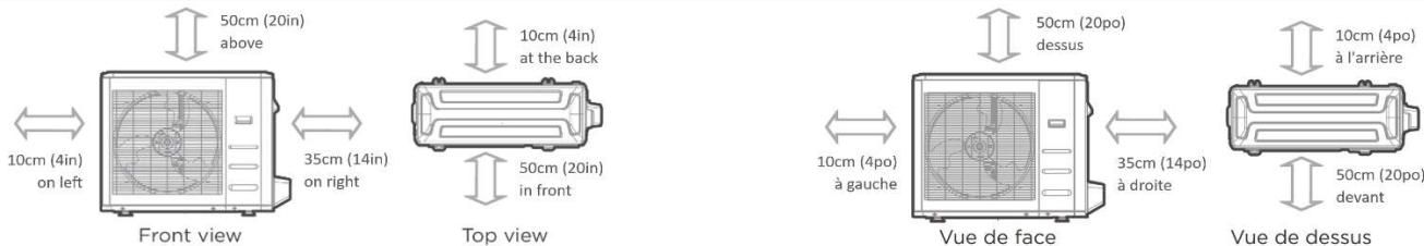
Note: Outdoor units must be elevated 30.5-61cm (12-24in.) above the surface below in heating applications to allow for snow clearance and defrost runoff. Follow local codes, best practices, and guidelines. Diagrams for reference only.
